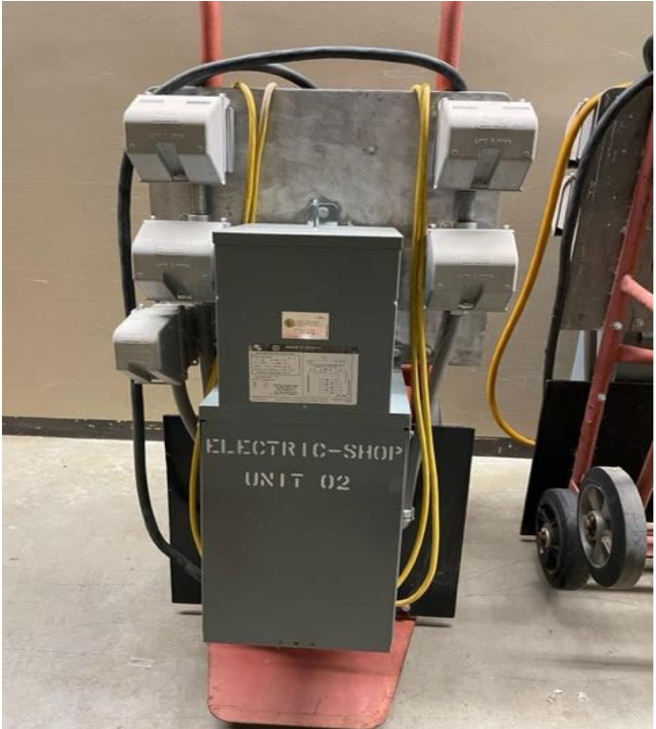
**Photo B** – Step down transformer from 480V to 120V
